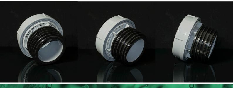
FloPlast's External Air Admittance Valve will allow the installation of an external soil pipe within 3 metres of any opening. It terminates at the same height as if it were installed internally, i.e. 200mm (minimum) above the highest wet entry point to the soil vent pipe. See diagram opposite.
