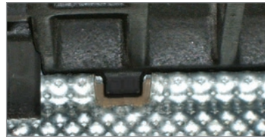
The anti-shunt lines the grate up to the channel and prevents the grates ability to move linearly. When cutting channels to required lengths, remember to also align the grate to the channel so the anti-shunt engages
