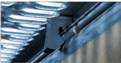
ACO Drainlock™ locking mechanism fastens into the channel. Gratings should be fitted in the channels before the installation concrete is installed
