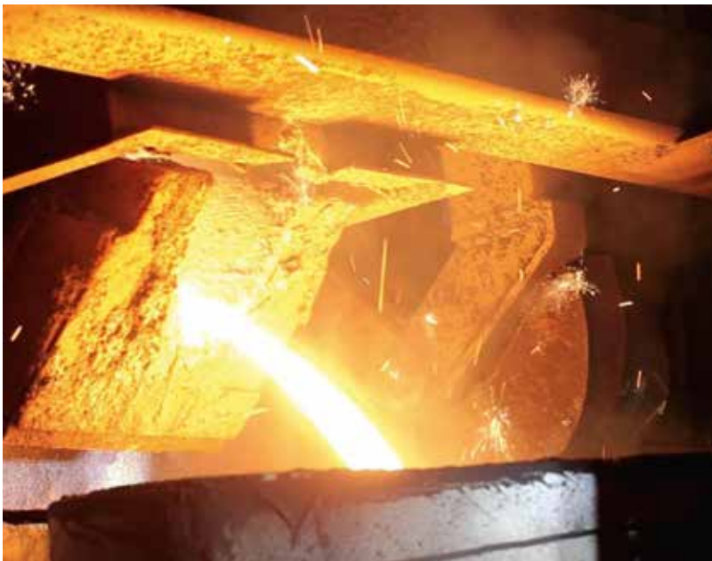
Molten cast iron in an electric furnace
