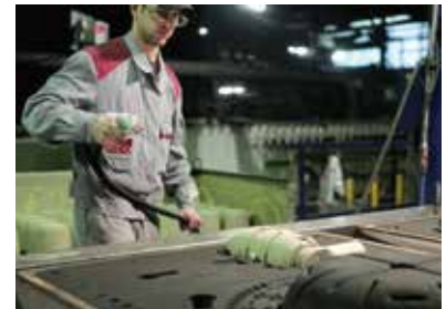
Insertion of the sand core
