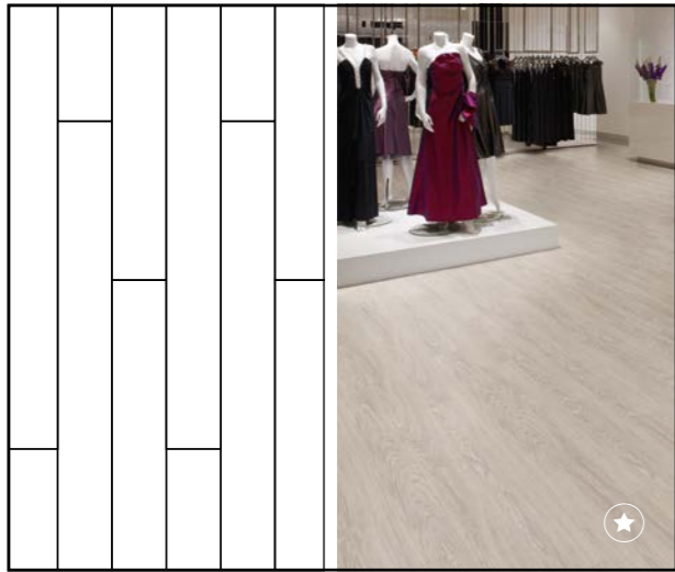
Straight laid plank - staggered
