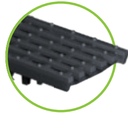
ductile iron elongated bar grating MW 29/13, class C or D for NW 100 to 200
