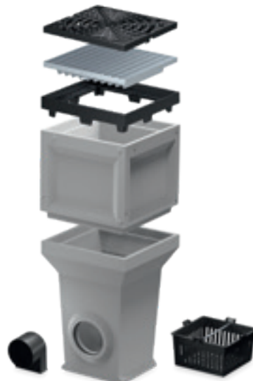
spot incl. cast iron frame with mesh grating or ductile iron grating up to class B incl. odour trap and sediment bucket extension-element optional
