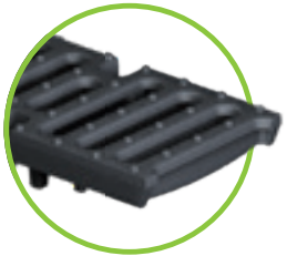
ductile iron slotted grating SW 14/100, 14/150, 14/200 for NW 100 to 200 class E, with fiX-locking for NW 150 to 200, class D, 4 point bolted
