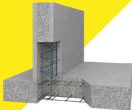
Base plate joints
