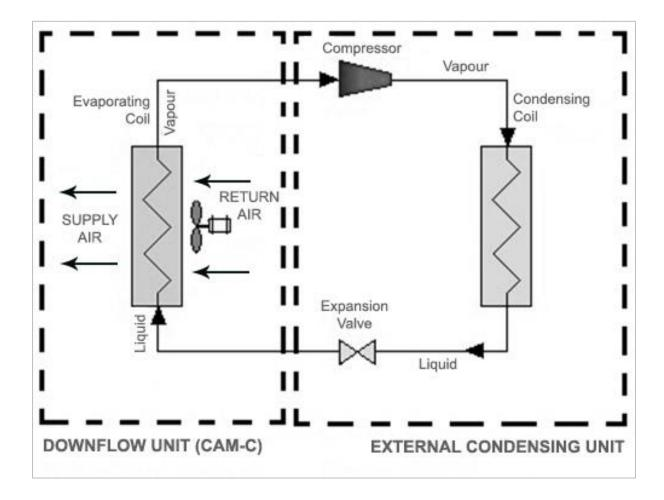
Typical coil selections are made for R410a refrigerant. In the event of high external temperatures, it is recommended to use R134a refrigerant, in which case the number of rows and pipe connections could change.
