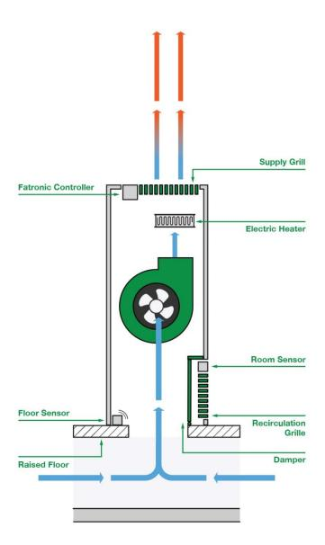
**Note**: A 5% reduction in airflow must be allowed when the TUC-500 is fitted with an optional electric heater.
