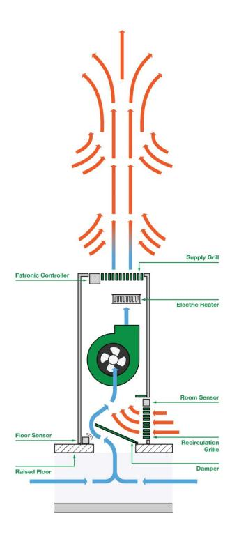
Note: A 5% reduction in airflow must be allowed when the TUC-500 is fitted with an optional electric heater.
