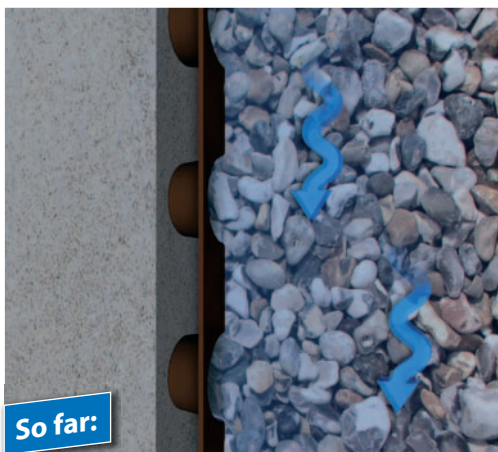
Dimpled sheet without drainage function – intruding water cannot easily drain away.
