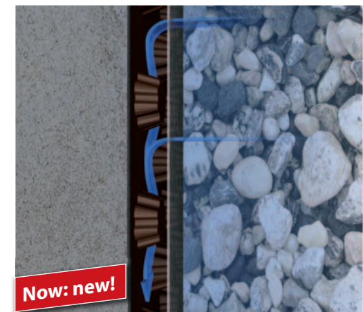
Through its high-performance drainage function, DELTA®-MS DRAIN offers an optimum escape for intruding water.
