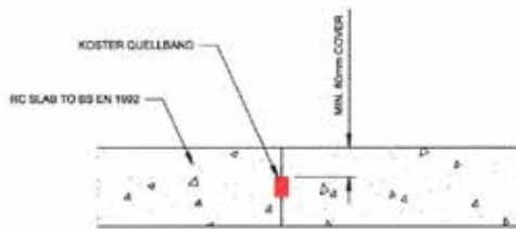
NEW SLAB CONSTRUCTION JOINT
