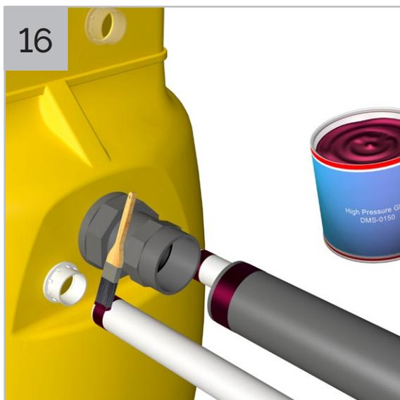
Apply Delta Solvent Cement around the first 20 mm of the external face of the discharge and cable duct pipe and internal side of their respective fittings.
