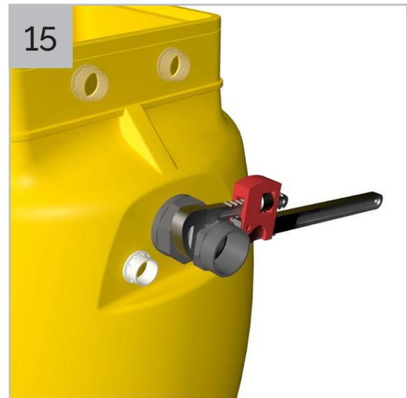
Securely fasten the plain/threaded socket onto the thread of the tank connector.
