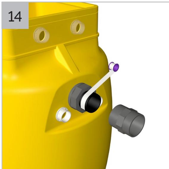
Wrap the thread on the tank connector's male thread with PTFE tape.
