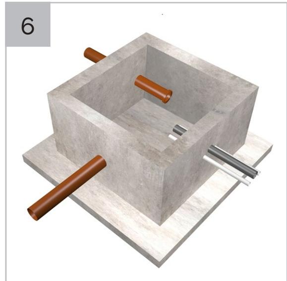
Allow the concrete to cure and then remove the shuttering.
