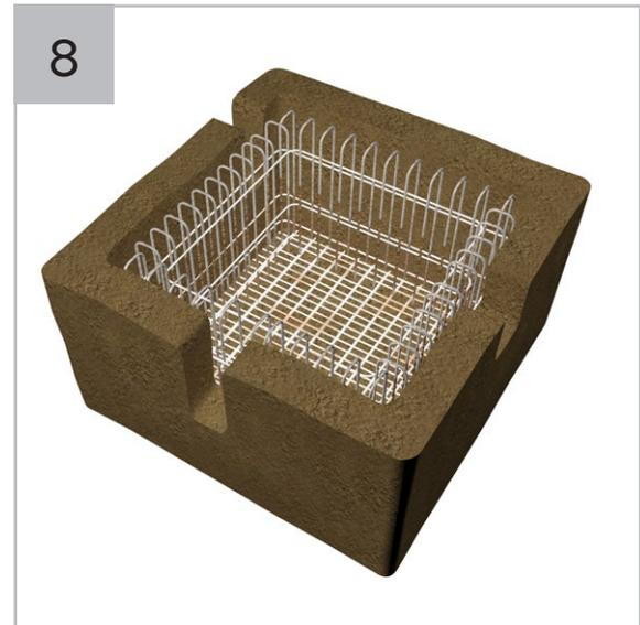
Install re-bar as per structural engineer's details.
