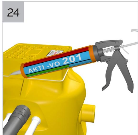
24 Once chamber has been filled with water, apply Delta AKTI-VO 201 (swellable mastic) to the entire external lip locator of chamber.
