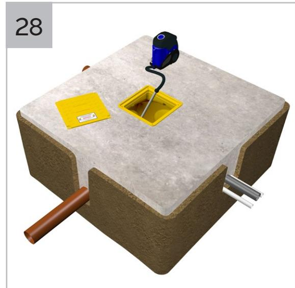
Manually remove any debris from chamber and residual water using a wet vacuum.
