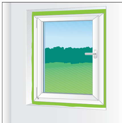
Fig 1 For the perimeter sealing of windows & doors
