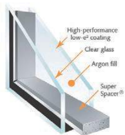
Illustration of a double glazed unit
