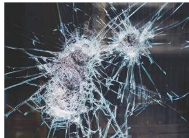
Laminated glass, retains the overall integrity of the glass.
