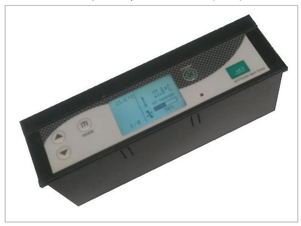
With the LCD controller, all programming setup and modification of the working parameters are carried out using the controller's four push buttons as indicated in the image above. The functions available depend upon the TU4 configuration; please refer to the Fatronic user manual for full information.
