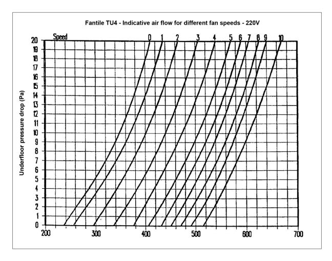
In the reading of the air flow value it must be considered that in a typical installation the under floor static pressure in the supply zone is normally between 3 and 15 Pa.
