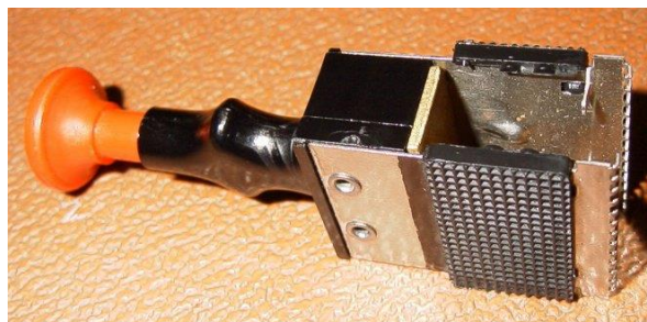
Figure 4 – Eprom (top) and Eprom Remover Tool
