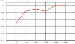
Gedina D/A 15 mm, 200 mm o.d.s.o.d.s = overall depth of system
