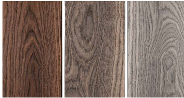
At Installation 6 months + 1 Year +
