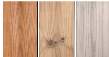
At Installation 6 months + 1 Year +
