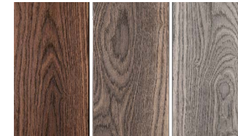
At Installation 6 months + 1 Year +
