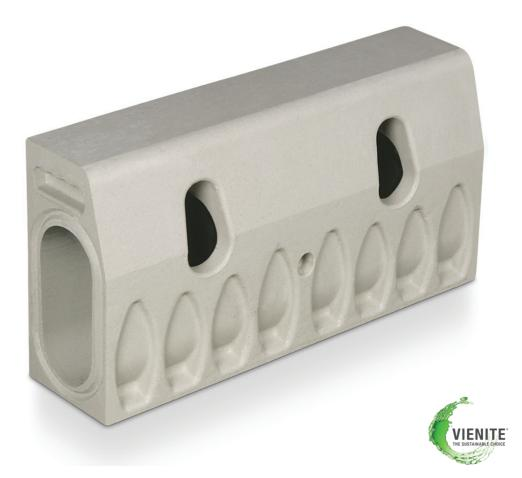
The ACO KerbDrain® 255 half battered range has a compact size to match a standard HB2 kerb stone. The range is ideal for smaller catchment areas or as a retrofit option in existing kerb installations where drainage or ponding in the highway is a problem.
