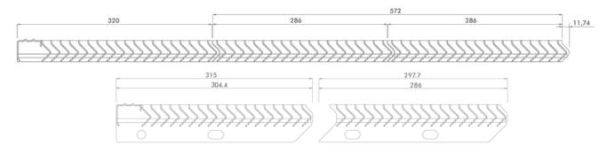
Flooring panels are framed either with a 34x4mm flat bar for laying on a steel section support or with a 60x4mm flat bar for side bolting.
