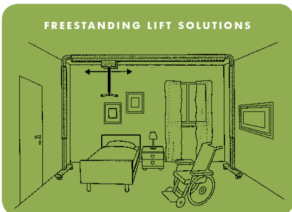
FreeStand is a sturdy and economical system for lifting on a straight rail.
