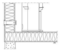
Indirect air supply through the external wall.
