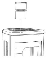
Make sure that the connector gasket does not work loose when the connection pipe is placed on the connector. If further sealing material is required, heatresistant sealant may be used.
