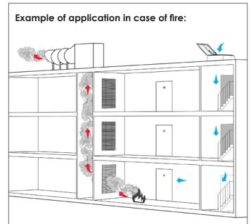
Damper opens and fan starts. The smoke and gas is drawn up and out via the exhaust duct.
